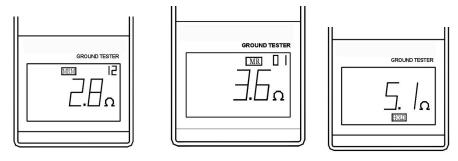
enters into reading mode, as shown in the figure in the right. At such momoent, the upper right corner of the screen shows the position of a record in the memory. Each time when the meter is in reading mode, the first record will be displayed first, and each short push (less than 3 seconds) on the HOLD button will make the next record displayed. After reading all 30 records, the first record will be displayed.
